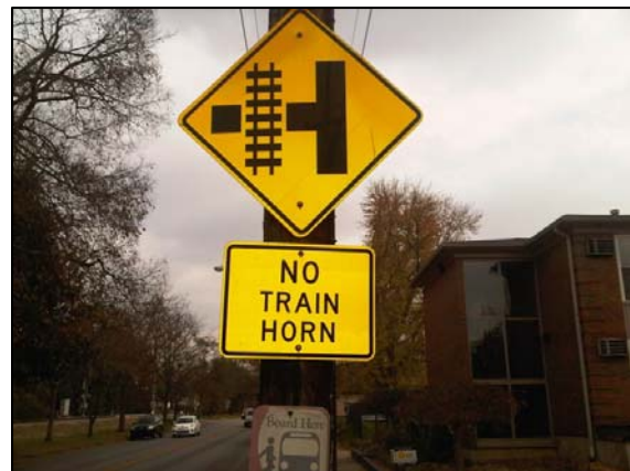
Quiet Zone Signage Located in Louisville, KY Photo by Parsons Brinckerhoff, 2014
